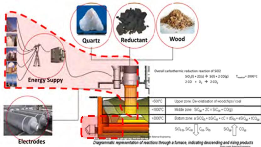
Figure 2. Typical raw materials and electricity path through electrodes in Si process (Viridis.iQ GmbH).
