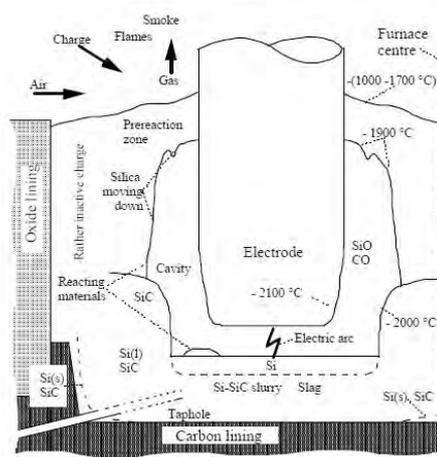
Figure 3. Distribution of phases and elements inside a silicon furnace. Liquid silicon in contact with carbon or SiO<sub>2</sub> may react and lower the productivity of the furnace, impacting the tapping process (Schei, Tuset, and Tveit, 1998).
