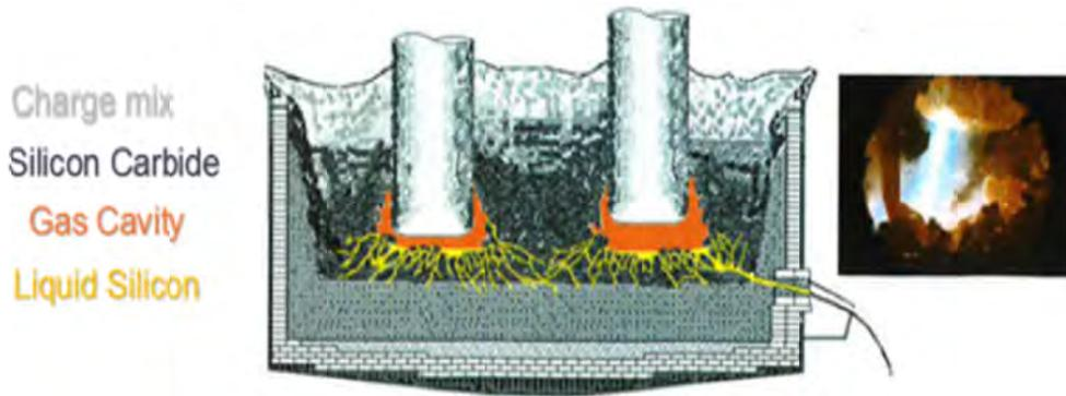
Figure 10. Schematic of a silicon furnace and photograph of crust build-up around gas cavity (Elkem report).
