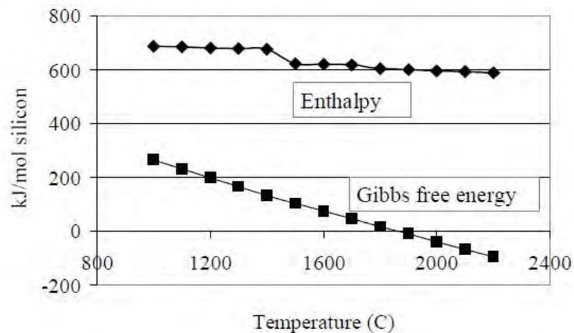
Figure 11. Thermodynamic parameters of the reverse reaction.
