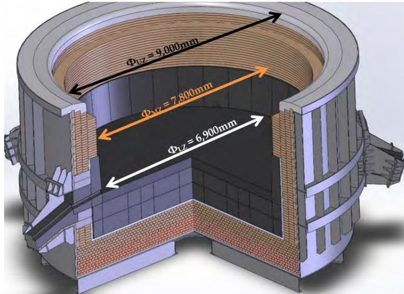
Figure 8. Schematic view of a submerged arc furnace shell used as a base case scenario (Viridis.iQ GmbH).
