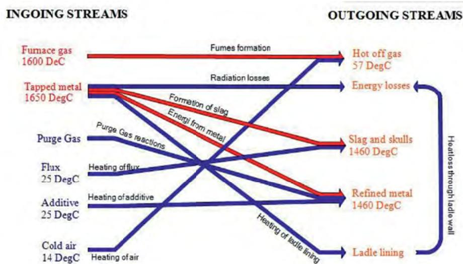
Figure 12. The energy streams in the tapping area (Kamfjord, 2012).
