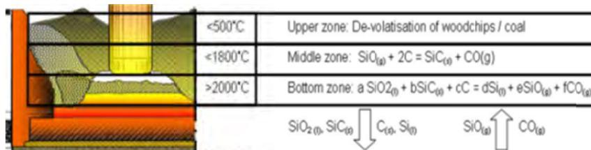
Figure 4. Diagrammatic view - reactions in a submerged arc furnace for silicon production (Bateman Engineering).
