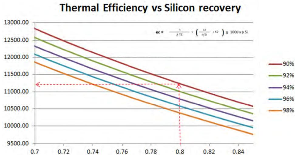
Figure 7. Silicon recovery vs thermal efficiency in metallurgical silicon manufacturing process (Schei, et al, 1998).
