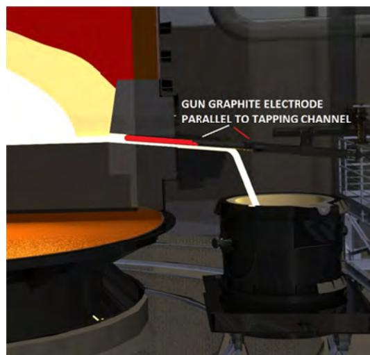
Figure 5. Cross-section of tap-hole and furnace hearth. The ladle, shell, furnace platform, and tapping tools are also depicted (Viridis.iQ GmbH).
